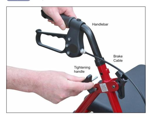
Insert the handlebar into the tubing ensuring the brake cable is to the outside of the rollator frame.
