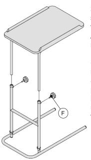
3. Connect the two sections of the table together as shown. Adjust the tabletop to the required height and angle. Insert the two handscrews (shown by 'F') into the receivers in the frame. Secure the table in position by turning the two handscrews clockwise, until they lock the table tubing into position.
